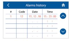
Each entry to the Alarms history contains the alarm/warning code and its date and time. The warning and alarm codes are detailed below.
