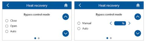
Depending on the particular AHU configuration use this window to select the necessary control mode for the bypass/rotary heat exchanger with discrete or analogue control.
