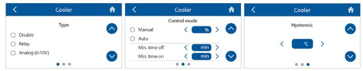
Select the cooler type (discrete/analogue) and its operation mode.
