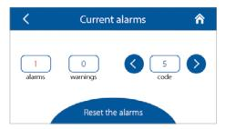
— number of current alarms. Indicates a serious malfunction. The unit is forced to shut down. The alarms must be reset manually.
