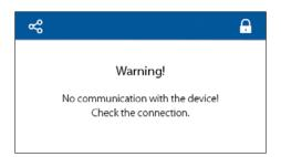
If the RS-485 network parameters are set incorrectly or if there is a problem with the cable, the display will show a warning ("No communication with the device. Check the connection").
