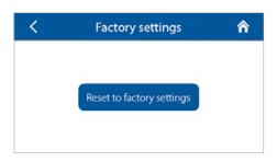
The reset may cause a temporary loss of connection to the device as it affects the Wi-Fi, RS-485 and Ethernet settings.
