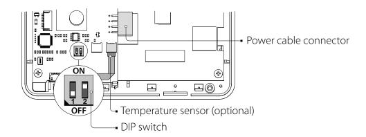
The temperature sensor is an optional device which measures the temperature in the room. If physically present in the panel configuration, select "Sensors in control panel" item in the control panel menu.
