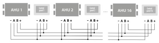
**Example 2** Connecting more than 5 control panels to a single AHU requires an external power supply unit.
