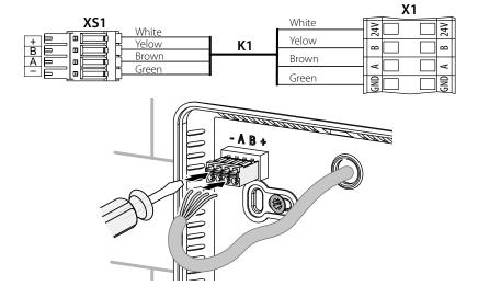
**5.** Remove the connector with the cable from the bracket and connect it to the female connector on the circuit board.
