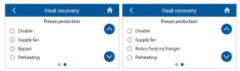
**Freeze protection** — type of heat exchanger freeze protection.
