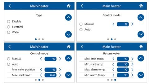
Select the heater type and set up its parameters.
