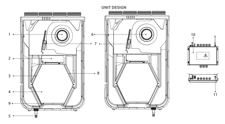
1 - exhaust fan; 2 - control unit (for VUT/VUE 270 V5(B) EC A2/A14 units); 3 - supply air filter; 4 - counter-flow heat exchanger; 5 - drain pipe (VUT 270 V5(B) EC); 6 - supply fan; 7 - bypass damper (only for VUT/VUE 270 V5B EC); 8 - extract air filter; 9 - drain pan; 10 - external control unit (for VUT/VUE 270 V5B EC A21 units); 11 - SETUP MODE button (for VUT/VUE 270 V5B EC A21 units).
