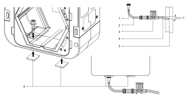
1 - drain pipe; 2, 4 - drain hose; 3 - U-trap; 5 - sewage system; 6 - additional insulation.
