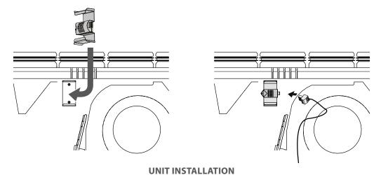
To attain the best performance of the unit and to minimize turbulence-induced air pressure losses, connect the straight air duct section to the spigots while installing.
