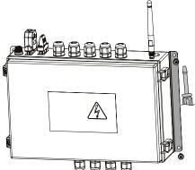
Design of hinges allows to change the opening side of a control unit cover. Unscrew the fixing screws, open the cover and unhinge it. Fix the cover to the opposite hinges, tighten the fixing screws.
