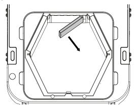
Access to the control unit VUT/VUE 270 V5(B) EC A2/A14
