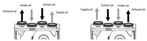
Make sure of the correct unit service side selection. Unit mounting position should enable free excess to the opening plate for maintenance and service operations. The plate opposite to the service side must be fixed with screws (included in the delivery set).
